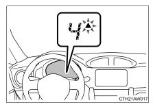
To help enable fuel-efficient driving, the shift-up indicator flashes 3 times to indicate upshift timing.
