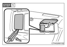
Open the cover and remove the lens.
