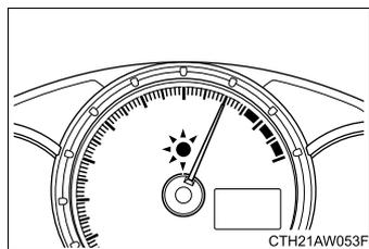
When the set engine speed is reached the REV indicator comes on and a buzzer sounds to inform the driver. (→P. 199)
