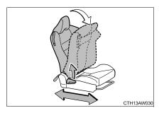
Lift the seatback angle adjustment lever.
