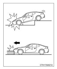
Only the driver's SRS frontal airbag or both driver's and front passenger's SRS frontal airbags may be activated when the vehicle sustains a hard impact in the undercarriage area from the road surface (such as when the vehicle plunges into a deep ditch, is severely impacted or knocked hard against an obstacle on the road such as a curb).
