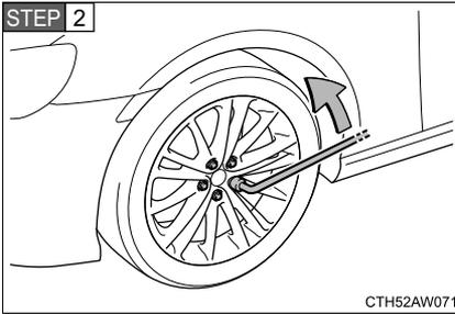
Slightly loosen the wheel nuts (one turn).
