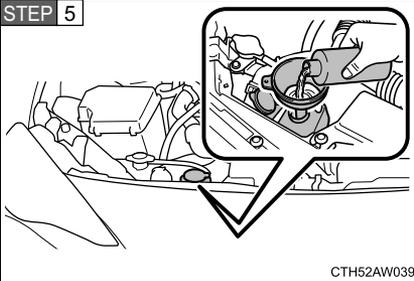
Add engine coolant if necessary.
