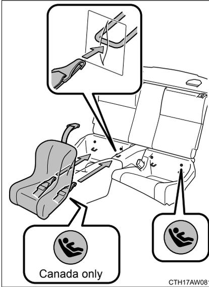
**STEP 1** Latch the hooks of the lower straps onto the LATCH anchors.
