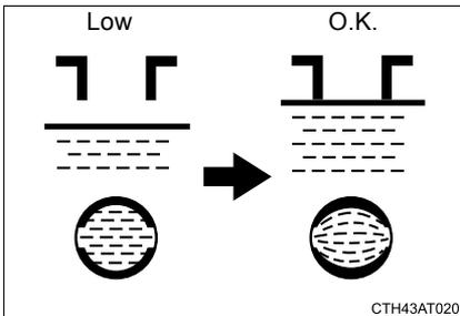
**STEP 1** Remove the vent plug.
