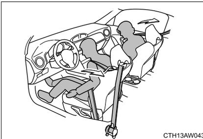
The pretensioner helps the seatbelt to quickly restrain the occupant by retracting the seatbelt when the vehicle is subjected to certain types of severe frontal collision and/or side collision.
