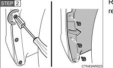
Remove the clips and partly remove the fender liner.
