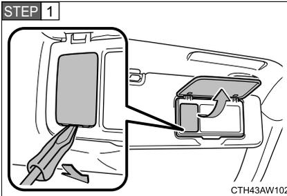
Open the cover and remove the lens.
