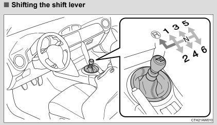
Fully depress the clutch pedal before operating the shift lever, and then release it slowly.
