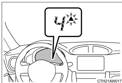
To help enable fuel-efficient driving, the shift-up indicator flashes 3 times to indicate upshift timing.
