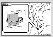
Pull the engine hood release lever.
