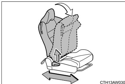
Lift the seatback angle adjustment lever.
