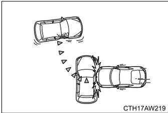
The vehicle strikes an object that can move or deform, such as a parked vehicle.
