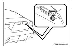
Turn the mechanical key clockwise to open.
