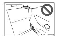
Always make sure that the seatbelt is not caught in the seatback or twisted in one of the hooks that secure the seatback. Failure to do so may cause the seatbelt to not be fastened correctly or to become ineffective in a collision, resulting in serious injury. 1
