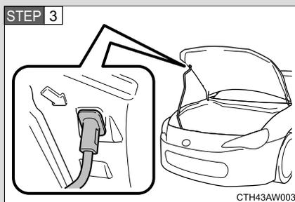
Hold the engine hood open by inserting the supporting rod into the slot.
