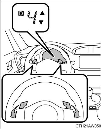
Temporary manual mode driving can be changed to by operating the paddle shift levers while the select lever is in the D position.
