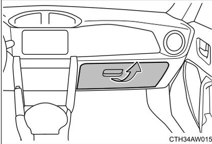
Pull up the lever to open the glove box.
