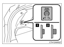
Turn the main switch in the trunk lid off to disable the trunk lid opener.
