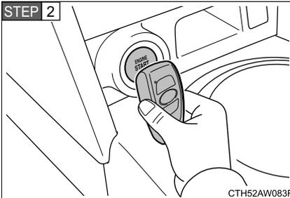
Touch the area behind the lock button and unlock button on the access key to the push-button ignition switch.
