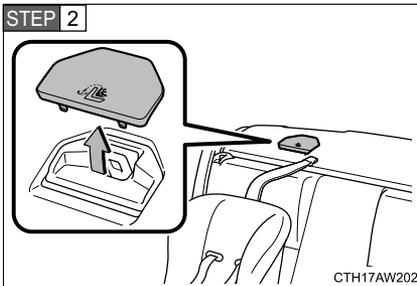
Remove the anchor bracket cover.
