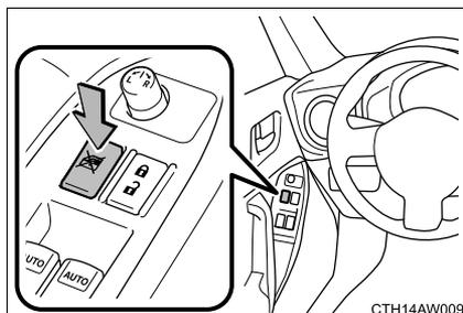
Press the switch down to lock the passenger window glasses.
