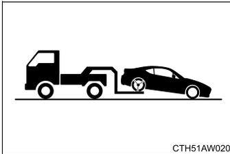
Ensure that the front lower body components have adequate clearance to prevent contact with the road surface under all conditions.
