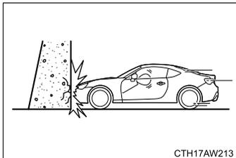
A head-on collision against a thick concrete wall at a vehicle speeds of 12 to 19 mph (20 to 30 km/h) or higher activates only the driver's SRS frontal airbag or both driver's and front passenger's SRS frontal airbags. The airbag(s) will also be activated when the vehicle is exposed to a frontal impact similar in fashion and magnitude to the collision described above.
