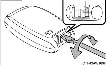
Insert the tip of a flathead screwdriver into the groove and remove the cover.
