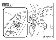
Open the driver's door while pressing and holding in on the power door lock switch and continue to press in for approximately 10 seconds after the driver's door has opened.
