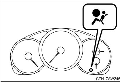
A diagnostic system continually monitors the readiness of the SRS airbag system (including front seatbelt pretensioners) while the vehicle is being driven. The SRS airbag system warning light will show normal system operation by illuminating for approximately 6 seconds when the ignition switch is turned to the “ON” position.
