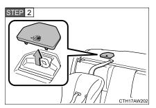
Remove the anchor bracket cover.
