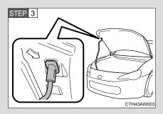
Hold the engine hood open by inserting the supporting rod into the slot.
