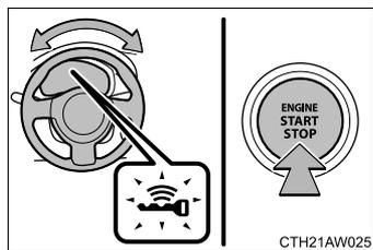
The keyless access with push button start system indicator light (green) will flash quickly.
