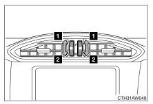
1 Open the air outlet. 2 Close the air outlet.
