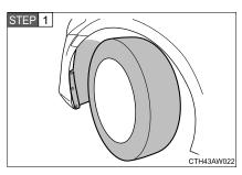
Turn the steering wheel in the opposite direction of the light to be replaced.
