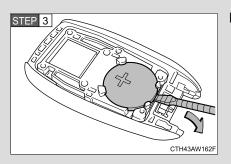
Remove the depleted battery.
