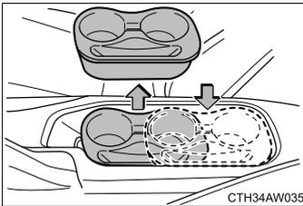
Remove the cup holder and change the holder position.
