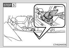
Add engine coolant if necessary.
