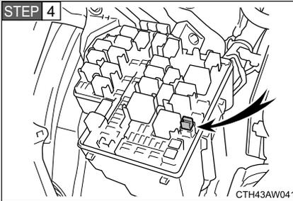
Remove the fuse with the pull-out tool.
