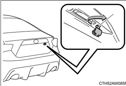
Turn the mechanical key clockwise to open.
