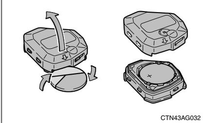
Open the case cover using a coin protected with tape and remove the depleted battery.
