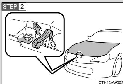
Push the auxiliary catch lever to the left and lift the engine hood.
