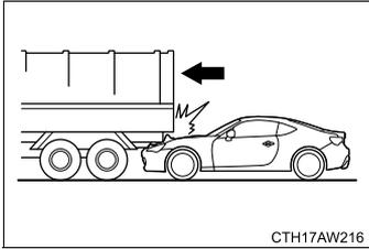
The vehicle slides under the load bed of a truck.
