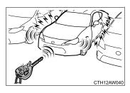
A buzzer (sounds once) and the hazard warning flashers (flash 3 times) are used to inform the driver of the vehicle's location.
