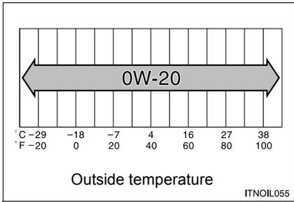
SAE 0W-20 is the best choice for good fuel economy and good starting in cold weather. If SAE 0W-20 is not available, SAE 5W-20 oil may be used. However, it must be replaced with SAE 0W-20 at the next oil change.
