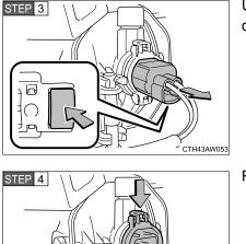
Unplug the connector while depressing the lock release.
