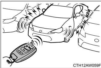
A buzzer (sounds once) and the hazard warning flashers (flash 3 times) are used to inform the driver of the vehicle's location.
