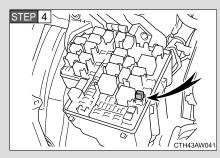
Remove the fuse with the pullout tool.
