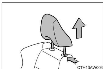
Pull the head restraint up while pressing the lock release button.
