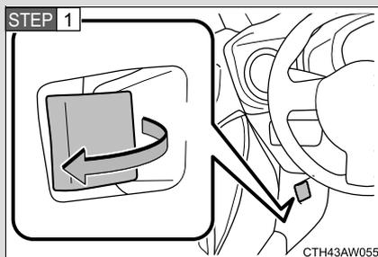
Pull the engine hood release lever.
