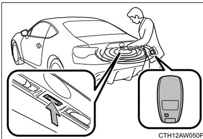
Press the button to unlock the trunk lid.
