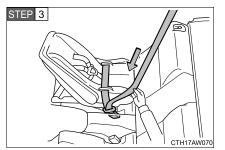
Fully extend the shoulder belt and allow it to retract to put it in lock mode. In lock mode, the belt cannot be extended.
