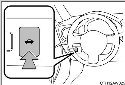
Press and hold the opener switch to release the trunk lid.
