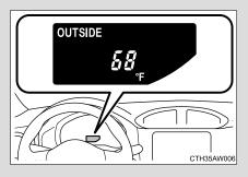
The outside temperature display can be switched by pressing the "DISP" switch.  $(\rightarrow P. 198)$
