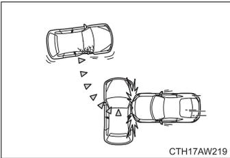
The vehicle strikes an object that can move or deform, such as a parked vehicle.
