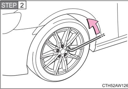
Slightly loosen the wheel nuts (one turn).
