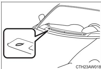
Headlight control sensor is located on the passenger's side.
