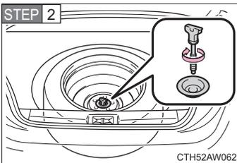
Install the center fastener as shown in the illustration.
