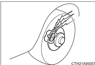
If you hear this scraping noise each time you apply the brake pedal, have the brake pads serviced by your SUBARU dealer as soon as possible.
