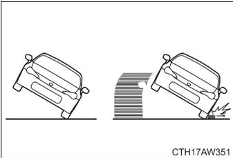
The side of the vehicle raises above a certain threshold or the vehicle skids and its tires hit a curbstone laterally.
