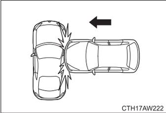
A severe side impact near the front seat activates the SRS side airbag and SRS curtain airbag.
