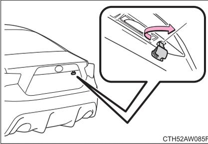
Turn the mechanical key clockwise to open.
