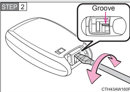
Insert the tip of a flathead screwdriver into the groove and remove the cover.
