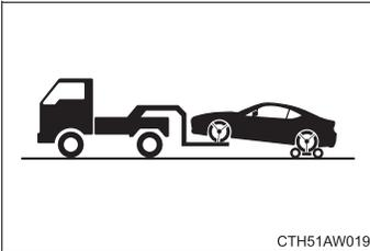
Never tow a vehicle from the front with the rear wheels on the ground. Use a towing dolly under the rear wheels.
