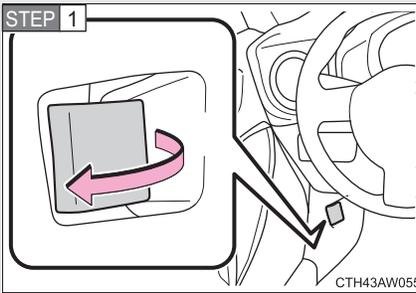
Pull the engine hood release lever.
