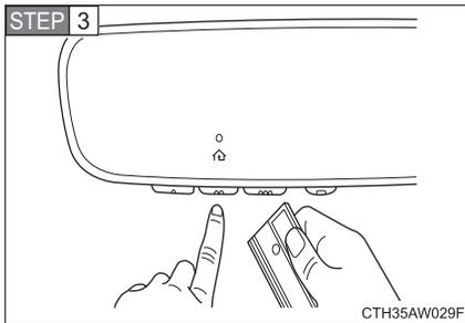
While the HomeLink indicator light is flashing orange, press and hold the hand-held remote button. Continue pressing the hand-held remote button until the HomeLink indicator light changes from orange to green. You may now release the hand-held remote button.
