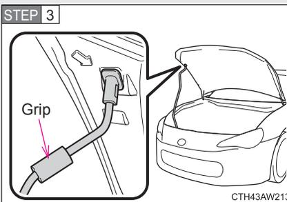
Hold the hood open by inserting the supporting rod into the slot.
