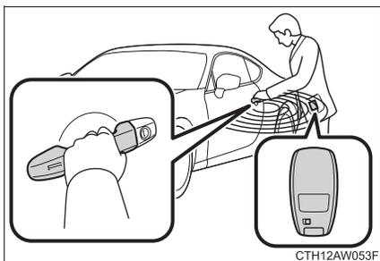
Grip the driver's door handle to unlock the door. Grip the passenger's door handle to unlock all the doors.
