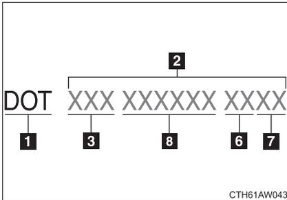
\*: The DOT symbol certifies that the tire conforms to applicable Federal Motor Vehicle Safety Standards.
