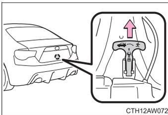
The trunk lid can be opened by pulling on the glow-in-the-dark lever located on the inside of the trunk lid.
