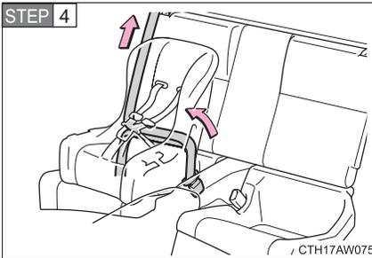
While pushing the child restraint system into the rear seat, allow the shoulder belt to retract until the child restraint system is securely in place.
