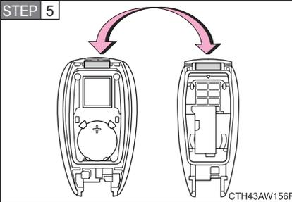
Align the protruding part with the slot and install the cover.
