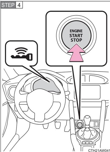
Press the push-button ignition switch shortly and firmly.
