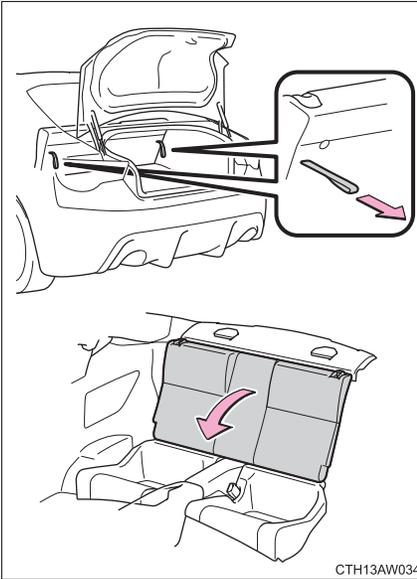
Pull the both left and right seatback lock release straps in the trunk lid to fold down the seatback.
