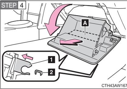
Lower the glove box slowly until surface **A** is horizontal with the floor, then pull it out. (Simply pulling with gentle force will disengage the lower claws.)
