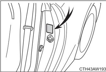
For the GAWR, see the Certification Label. For the maximum load of the tire, see the load limit at maximum cold tire inflation pressure mentioned on the sidewall of the tire. (→P. 502)
