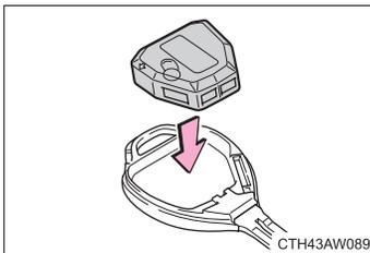
Insert the module from directly above. Inserting it on an angle may prevent the key buttons from operating properly.
