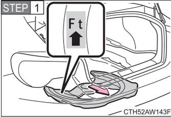
Vehicles with a T145/70D17 compact spare tire only: Install the spare tire spacer with the “Ft↑” mark facing the front of the vehicle and the rear edge of the spacer contacting the vehicle body.
