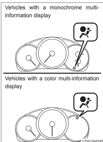
A diagnostic system continually monitors the readiness of the SRS airbag system (including front seatbelt pretensioners) while the vehicle is being driven. The SRS airbag system warning light will show normal system operation by illuminating for approximately 6 seconds when the ignition switch is turned to the “ON” position.
