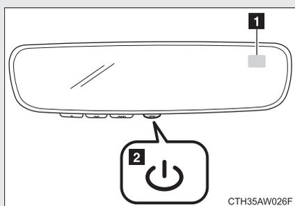
To turn the compass feature on/off, press and hold the
