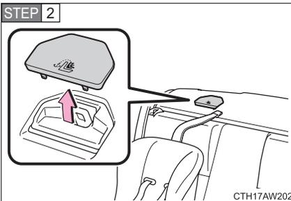
Remove the anchor bracket cover.
