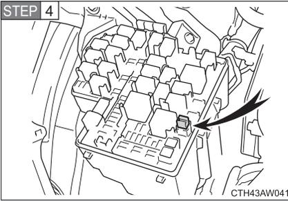
Remove the fuse with the pull-out tool.
