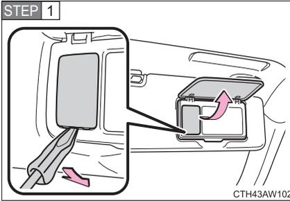
Open the cover and remove the lens.
