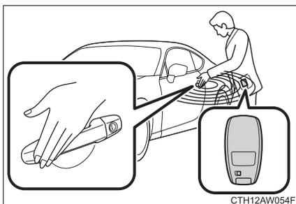
Touch the lock sensor (the indentation on the side of the door handle) to lock the doors.
