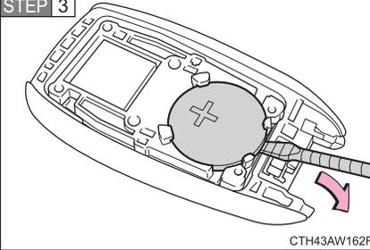
Remove the depleted battery.
