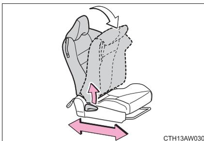
Lift the seatback angle adjustment lever.
