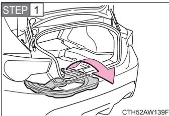
Vehicles with a T145/70D17 compact spare tire only: Before stowing the flat tire, remove the spare tire spacer.
