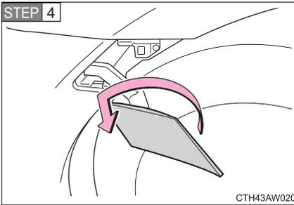
Pull out the lamp and turn the lens counterclockwise.
