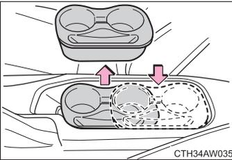
Remove the cup holder and change the holder position.
