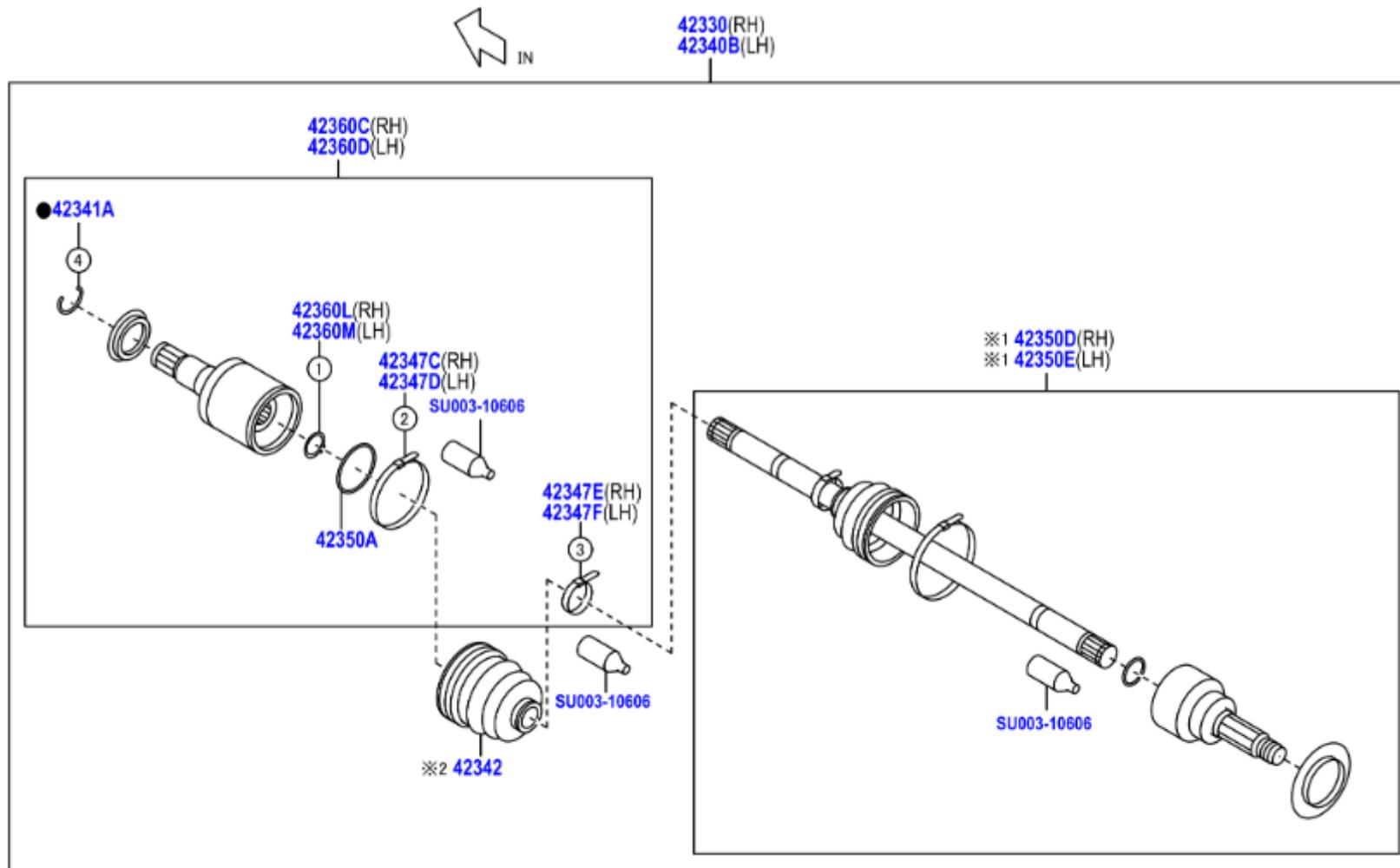
※1 PNC 42350D(RH),42350E(LH) does include ①,②,③,④ parts
